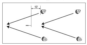
Figure 18: Measurement Mic Placement for Setting Delay
